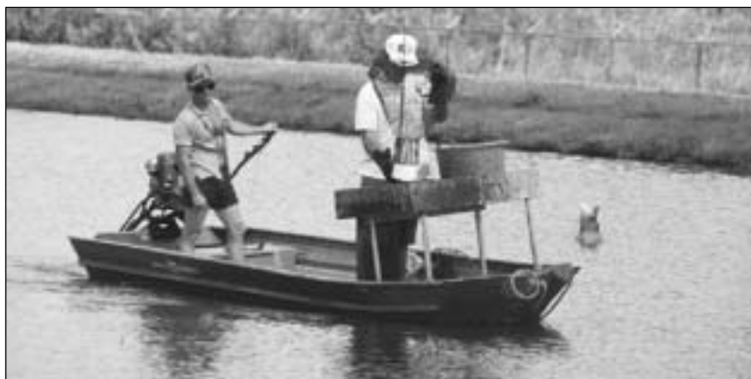
Figure 6. A crawfish harvesting boat powered by a Go-Devil propulsion unit (photo, LSU AgCenter).
